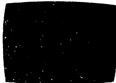
Example of playback with dirty video heads
